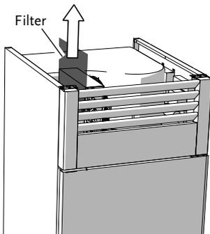
3. Clean the filter with a vacuum cleaner, wash with cold water, and shake off any excess water before refitting.
