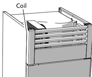
3. Brush the condenser coil with a soft brush to remove any dust or fluff.
