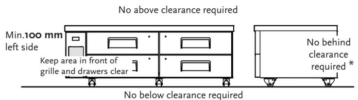
\*When installed for continuous duty in a climate class 7 environment (35°C ambient / 75% relative humidity), SKOPE recommends providing 50 mm clearance around the sides and back of the cabinet.
