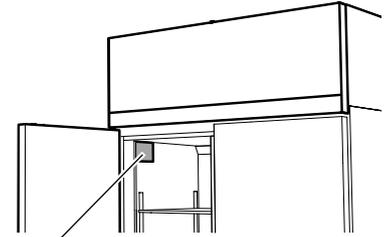
The rating label is located inside the cabinet at the top front of the left or right side wall.
