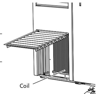
3. Brush the condenser coil with a soft brush to remove any dust or fluff.
