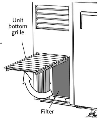
3. Clean the filter with a vacuum cleaner, wash with cold water, and shake off any excess water before refitting.
